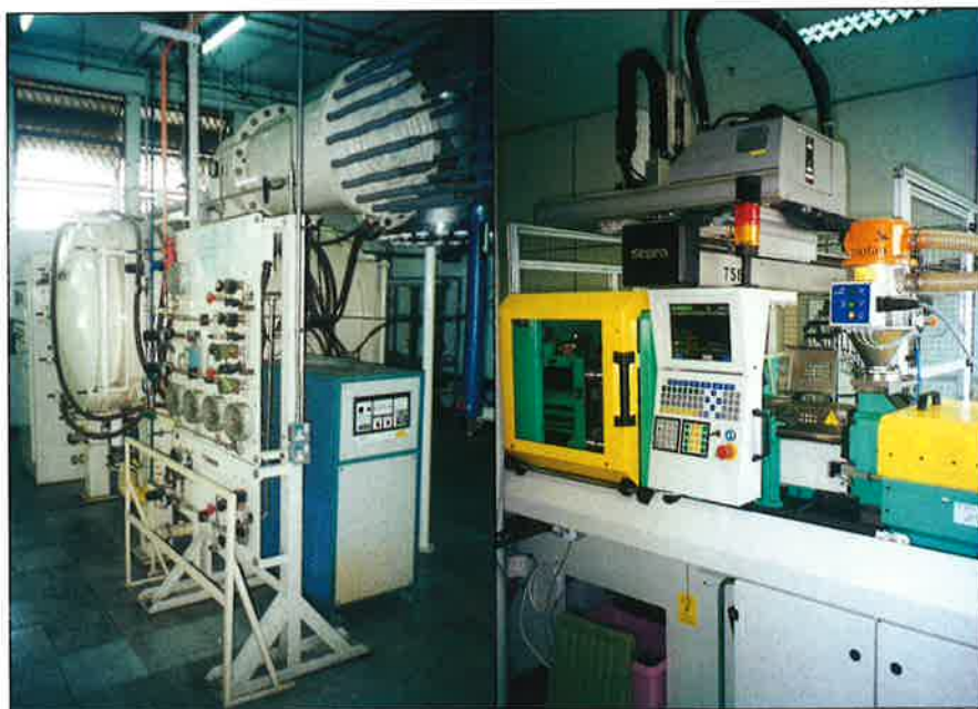
The sintering process makes use of high temperature furnaces to forge-produce the final shapes of the brackets
